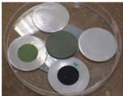
Button cells manufactured in-house
